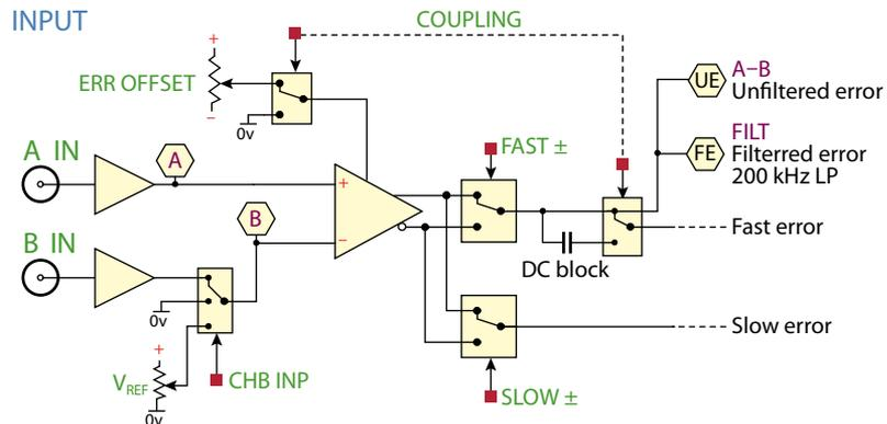
**Figure 1.5:** Schematic of the FSC input stage, showing coupling, offset and polarity controls. Hexagons are monitored signals available via the front-panel selector switches.
