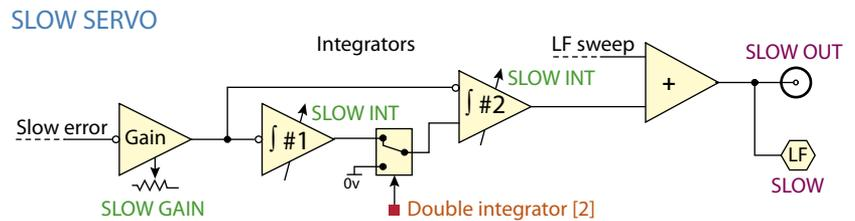
**Figure 1.6:** Schematic of slow feedback PI/PI<sup>2</sup> servo. Hexagons are monitored signals available via the front-panel selector switches.
