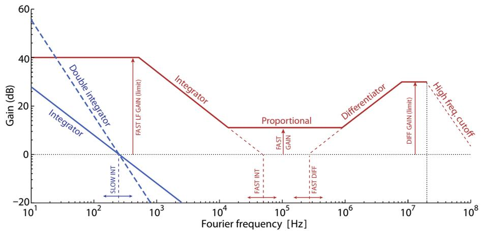
**Figure 1.3:** Conceptual Bode plot showing action of the fast (red) and slow (blue) controllers. The slow controller is either a single or double integrator with adjustable corner frequency. The fast controller is PID with adjustable corner frequencies and gain limits at the low and high frequency limits.
