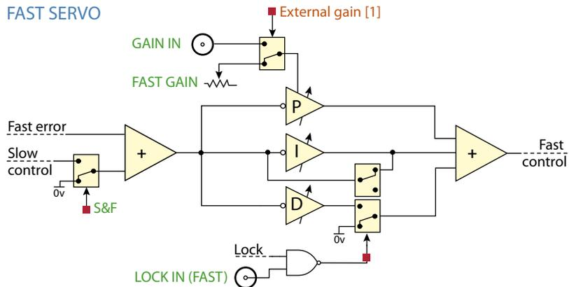
**Figure 1.7:** Schematic of fast feedback servo PID controller. Front panel controls for integrator and differentiator constants and limits are not shown.
