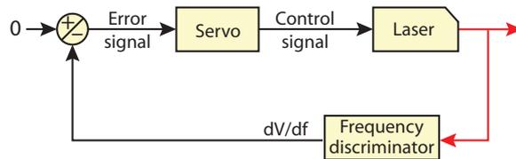
Figure 1.1: Simplified block diagram of the FSC.
