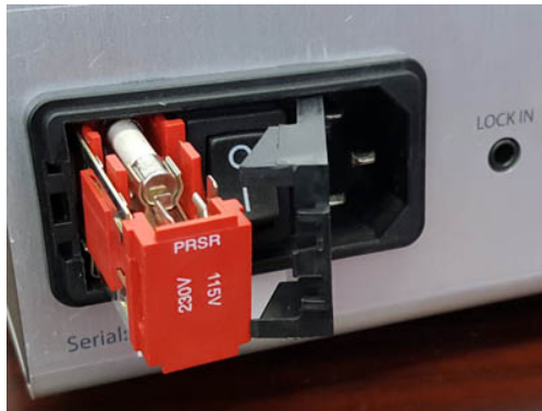
Figure B.1: Fuse cartridge, showing fuse placement for operation at 230 V.
