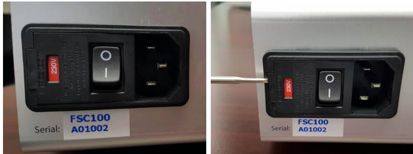
Figure B.2: To change fuse or voltage, open the fuse cartridge cover with a screwdriver inserted into a small slot at the left edge of the cover, just to the left of the red voltage indicator.
