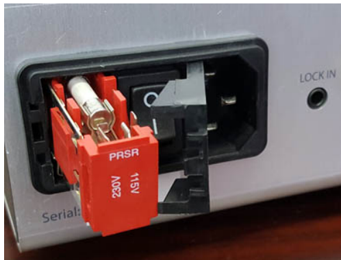
Figure E.1: Fuse cartridge, showing fuse placement for operation at 230Vac.
