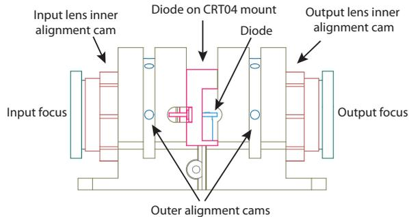
**Figure 2.1:** Eccentric cam sub-assembly.
