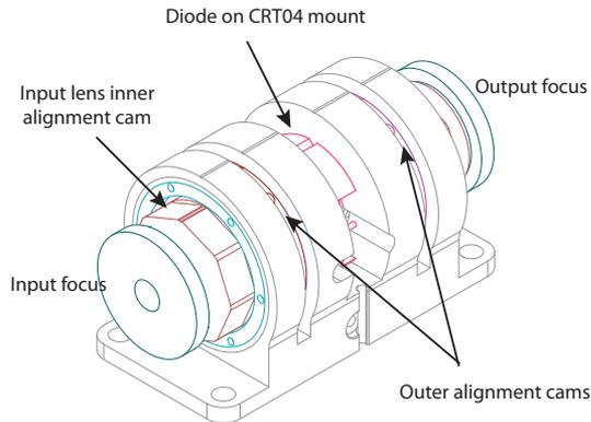
**Figure 2.2:** Eccentric cam sub-assembly.
