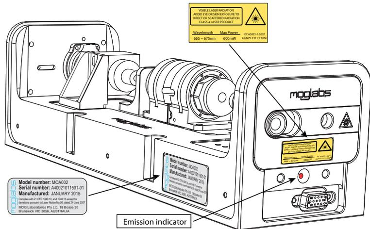
**Figure 2:** Schematic showing location of warning labels compliant with International Electrotechnical Commission standard IEC 60825-1:2007, and US FDA compliance label. Aperture label engraved on the front of the MOA002 near the exit aperture; warning advisory label on the rear and compliance label beneath.
