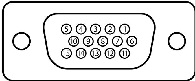
**Figure B.1:** Connector pinout. Relay (-) should be grounded to open the protection relay and enable operation.
