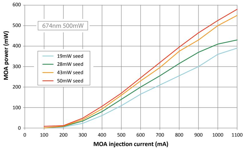
**Figure 2.5:** TA output against diode current, for several different injection seed laser powers (measured pre-isolator).
