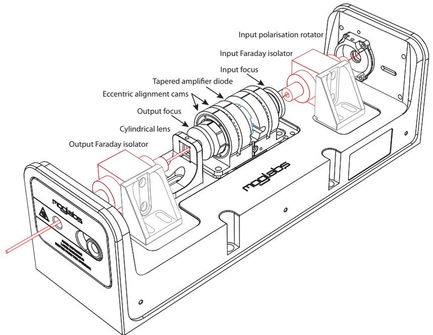
**Figure 1.1:** Schematic diagram of major components in the MOA002, including tapered amplifier diode, collimation lens eccentric cam alignment mechanism, cylindrical lens astigmatism compensator, Faraday isolators.
