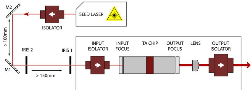
**Figure 2.3:** Alignment setup for aligning MOA002 to seed laser.
