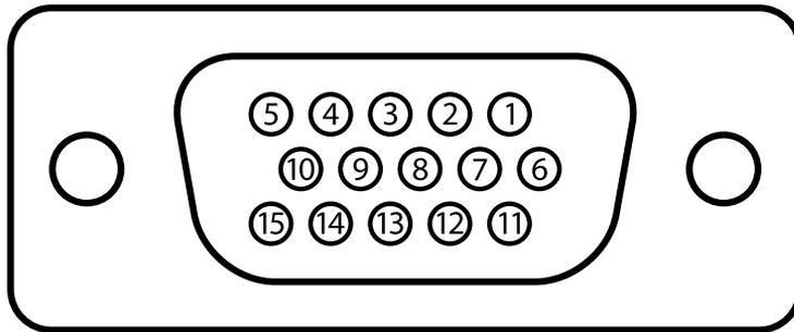
Figure B.1: Connector pinout. Relay (-) should be grounded to open the protection relay and enable operation.
