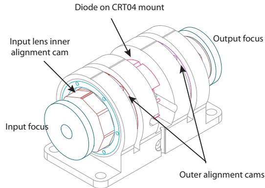
**Figure 2.2:** Eccentric cam sub-assembly.
