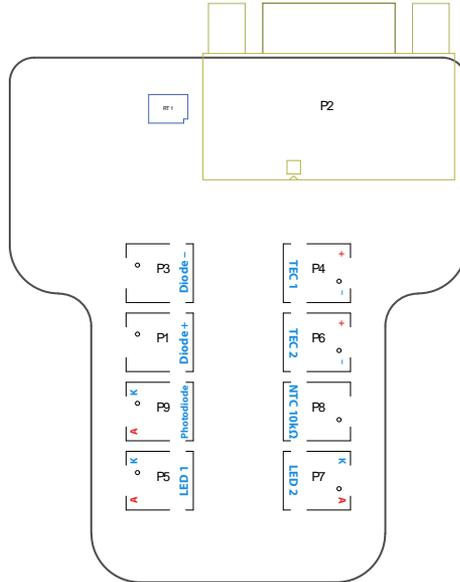
**Figure B.2:** MOGLabs MOA002 laser head board showing connectors for tapered amplifier diode, temperature sensor, TEC and LEDs.
