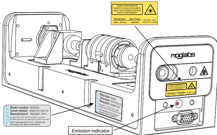
**Figure 2:** Schematic showing location of warning labels compliant with International Electrotechnical Commission standard IEC 60825-1:2007, and US FDA compliance label. Aperture label engraved on the front of the MOA002 near the exit aperture; warning advisory label on the rear and compliance label beneath.
