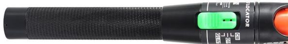
Figure 6.1: Fibre laser pen, or visual fault locator. Injects visible laser beam into fibre, which allows basic alignment and mode matching.
