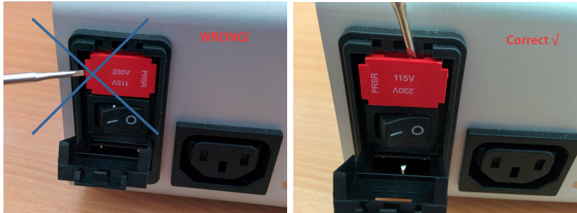
Figure M.3: To extract the fuse cartridge, insert a screwdriver into a recess at the top of the cartridge.
