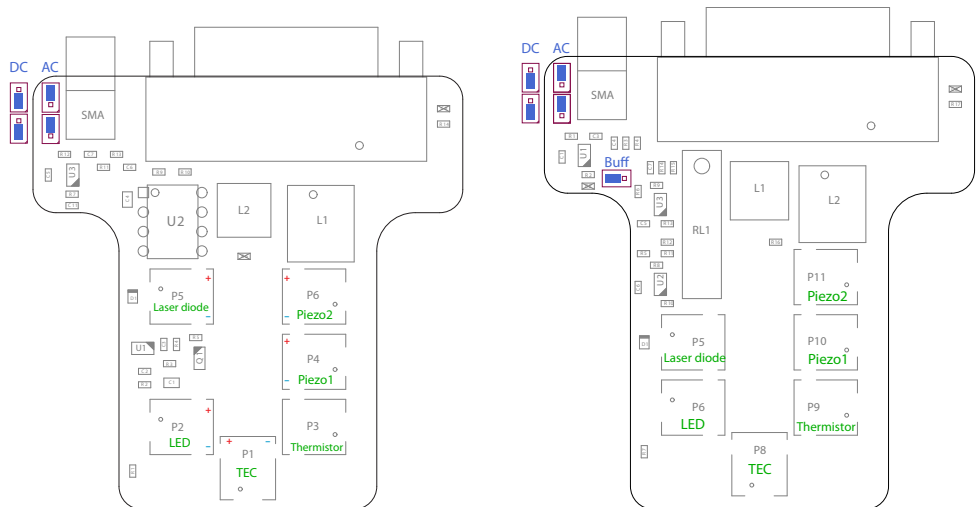
Figure I.4: B1047 (left) and B1240 (right) enhanced laser head boards. Jumpers at top left can be configured for AC or DC coupling. The B1240 has an additional jumper “Buff” for direct or buffered (differential) ground coupling, shown connected for differential coupling; change to pins 1 and 2 for direct. Modulation input via SMA connector, sensitivity 2.5mA/V. Connectors are Hirose DF59.
