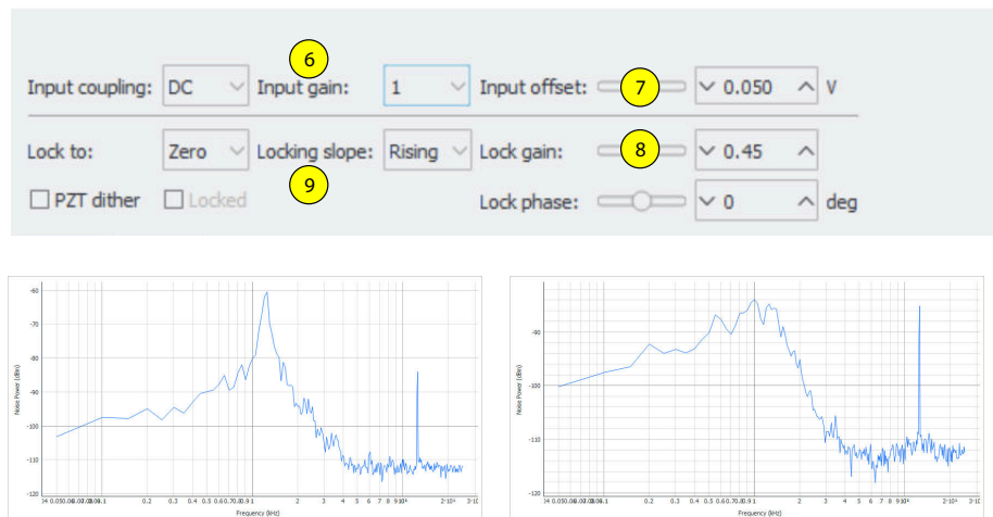
Figure 3.2: mLC locking controls: (6) input gain, (7) input offset, (8) lock gain, (9) locking slope, and error signal spectrum when the control loop gain is too high (lower left) and optimal (lower right).
